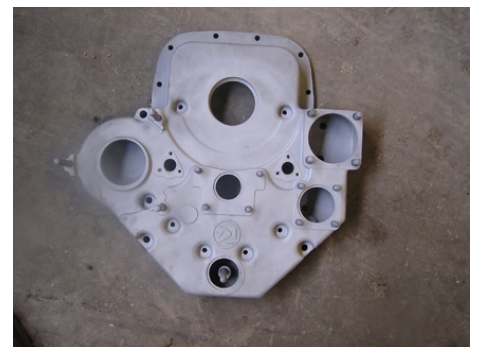
And new Kiekhaefer drive gear cover
