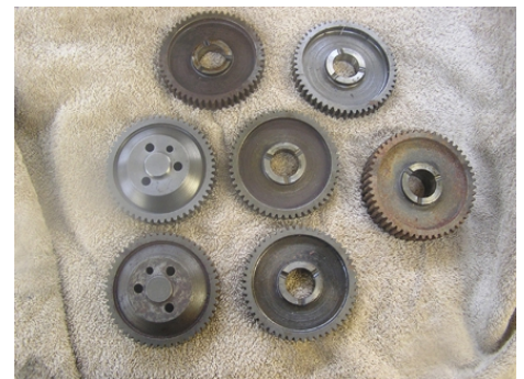
New Kiekhaefer accessory drive gears
